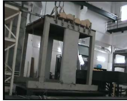
( b ) Retrofitted Specimen After Test
