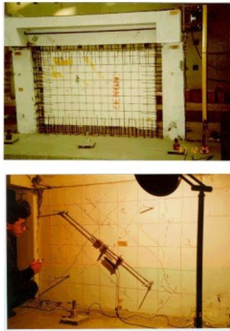
(a) Fabrication of Specimen and Tested Panel
